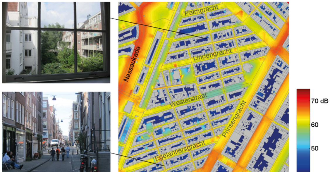
Figure 2.6. Part of the traffic noise map of Amsterdam from figure 2.4. There are busy streets (orange), less busy streets (yellow), quiet courtyards (blue) enclosed by houses (grey). The less busy streets, illustrated by the lower photograph, are typical of this lively urban area (Jordaan area). The upper photograph shows a view from a quiet façade on a quiet courtyard.
